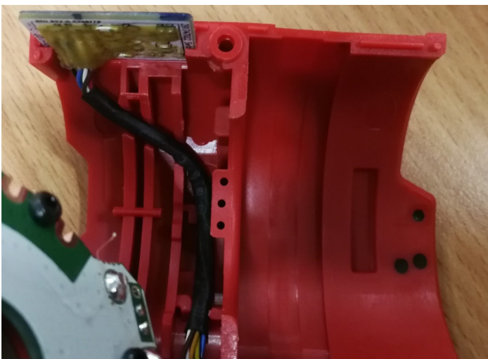
STEP 5: Install the pop switch into housing halve as shown. Route wires through traps being sure wires are tucked completely down.
